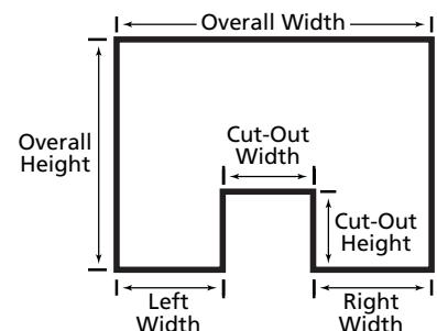
Measure a cut-out like a standard rectangular blind, but also provide detailed measurements of the area to be removed. In addition, mark the measurements on a sketch of the cut-out to ensure accurate communication of the order.
