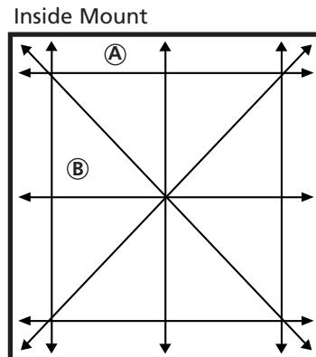
*With inside mounts, measure the width and height at three points and order the smallest dimensions.*
