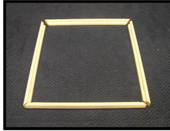
4. Position the left frame and the top frame onto a flat surface (small wood block is recommended to prevent damage to floor and to ensure a flush fit by the Hoffman Key) and line up the Hoffman key.
