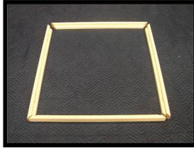
3. Position the left frame and the top frame onto a flat surface (small wood block is recommended to prevent damage to floor and to ensure a flush fit by the Hoffman Key) and line up the Hoffman key.
