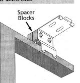
by 1/2"; use a maximum of three per installation bracket. Check that your mounting screws are long enough to securely attach the installation bracket and the spacer blocks. The solid side of the blocks should face the mounting surface. As with all outside mount installations, make sure the tops of the installation brackets are perfectly horizontal and aligned at the same height.
