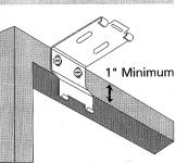
the locations you marked. Before tightening the screws, check to be sure the tops of the installation brackets are perfectly horizontal and aligned at the same height.
