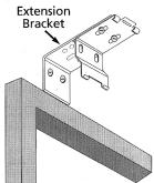
aligned at the same height. Connect the installation brackets with the machine screws and speed nuts which are included with each extension bracket. Be sure to use the same holes on all the extension brackets, so that each installation bracket projects the same distance from the mounting surface. Indentations are cast into the extension brackets between the holes. Before mounting an extension bracket, any unneeded length may be cut off at one of the indentations.
